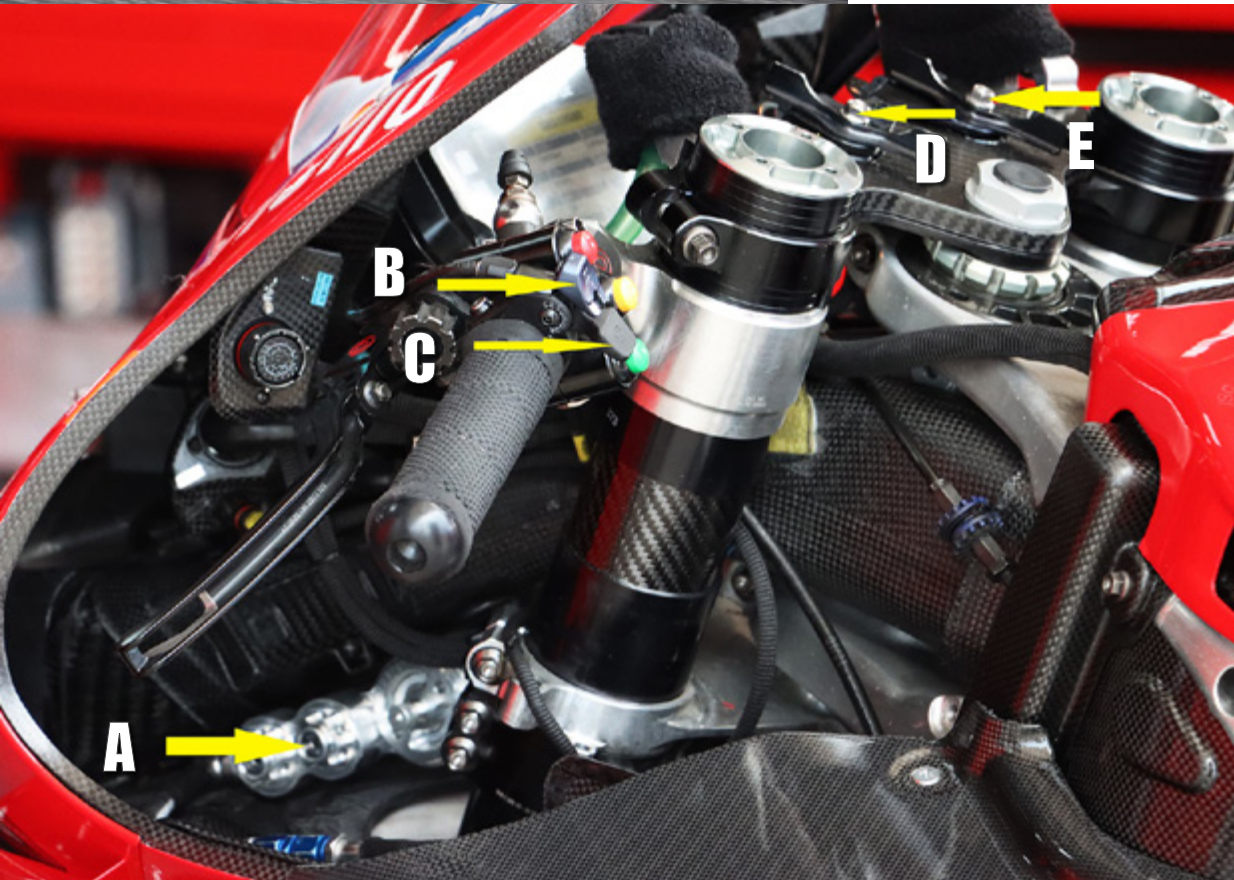
A close-up of a Ducati GP22 Desmosedici MotoGP Racebike’s ride height and holeshot device controls, taken just before a crew member intervened. (A) is the hydraulic unit. (B & C) are on/off ride height selector switches. (D & E) are hole-shot device selector levers for the front and rear suspension. Mat Oxley photo.
