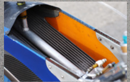
Rob Tuluie and the Tul-Aris at Willow Springs Raceway circa 2000, when he was 36. (Inset) The radiator is located horizontally in a tunnel that looks like a Meredith tube, which generates added thrust.
