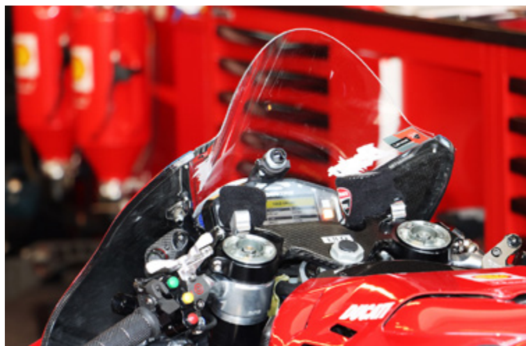
(Above) The Ducati GP23 holeshot system is controlled by silver lever on the left bar. (Above, Right) The GP23 mass damper is built into the tailsection. (Right) Accumulators seen at lower right are hydraulic pressure storage reservoirs. When the rider turns on the holeshot/ride-height system, pistons drop to displace damper fluid in the shock and lower the bike. Photos by Mat Oxley.
