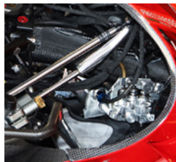
(Above) The Ducati GP23 holeshot system is controlled by silver lever on the left bar. (Above, Right) The GP23 mass damper is built into the tailsection. (Right) Accumulators seen at lower right are hydraulic pressure storage reservoirs. When the rider turns on the holeshot/ride-height system, pistons drop to displace damper fluid in the shock and lower the bike. Photos by Mat Oxley.
